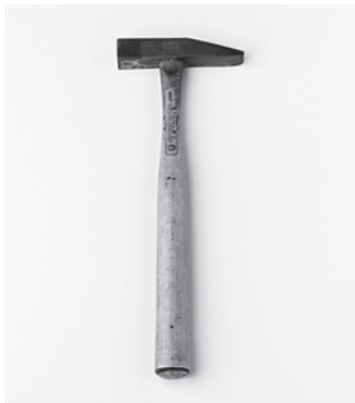
IMAGE SIXTEEN: The Stanley Works. USA, est. 1843. Stanley-Bostitch. USA, 1896. Tinsmith's Hammer. Before 1940. Steel and wood, 12 x 4 3 / 8 x 1" (30.5 x 11.1 x 2.5 cm). Purchase
