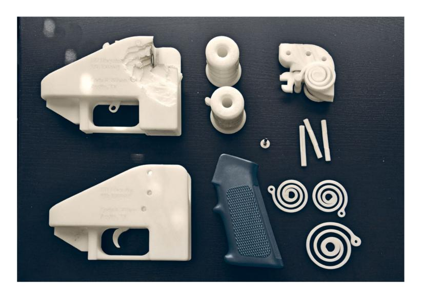
Partial components of The Liberator (clockwise from top left): ABSplus thermoplastic frame, barrel, hammer body, frame pins, springs, grip; aluminum nail (center)
