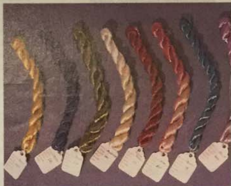
Closeup of Chardonnet artificial silk card (above, right), 1896, showing that undyed sample is in good condition, dyed sample has degraded; various colored skeins of viscose (right) made by Cross & Bevan, ca. 1914, in varying states of preservation (some faded, perhaps owing to strong light when displayed or dyes used); and woven Steam artificial silk samples (above), 1900s, that are fragile and discolored in places. Photos courtesy of Trustees of the Science Museum, London
