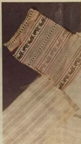
Closeup of Chardonnet artificial silk card (above, right), 1896, showing that undyed sample is in good condition, dyed sample has degraded; various colored skeins of viscose (right) made by Cross & Bevan, ca. 1914, in varying states of preservation (some faded, perhaps owing to strong light when displayed or dyes used); and woven Steam artificial silk samples (above), 1900s, that are fragile and discolored in places. Photos courtesy of Trustees of the Science Museum, London
