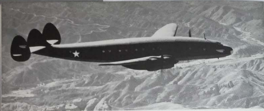
Lockheed Constellation. The largest land-based transport plane yet built, and the newest development for post-war commercial passenger use. Designed to carry 55 passengers, it is now being used as a troop carrier.
