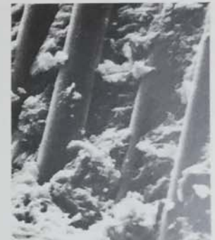
Electron microscope at 900X reveals homogeneous nature of Fibreglas reinforcement throughout an FRC panel.
