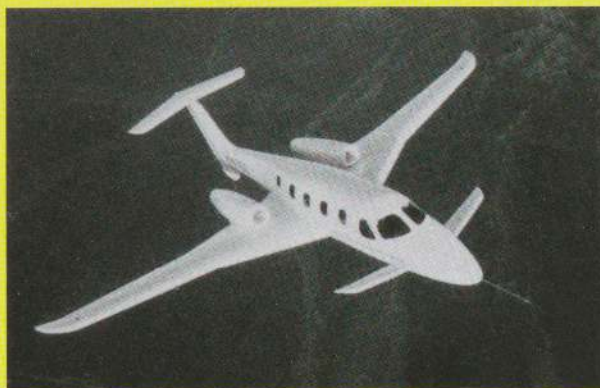
Burt Rutan, of Scaled Composites. "Triumph" Business Turbo-fan Twin-engine Plane. 1985–87 (tested 1988). Fiberglass and graphite in resin matrix, 19' 5" (6 m) x 48' (14.6 m). Prototype.
