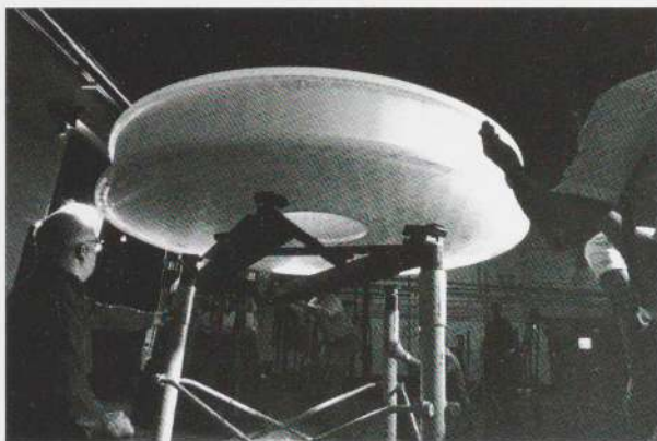
Figure 4. Corning Technical Products Division. Hubble Space Telescope Mirror Blank. 1990 (c. 1978). ULE glass, 8' (2.4 m) dia. Manufactured by Corning Incorporated, United States.
