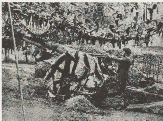
A WELL-CAMOUFLAGED ARTILLERY POSITION showing the use of overhead nets garnished with strips of painted canvas. The disruptive design on the canvas covering and the gun barrel conceal the form of the gun.
