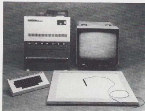
MCI/Quantel Paint Box digital art/graphics system. Enhancements shown at NAB include hundreds of new type faces, a "Font Factory" for entering custom faces and logotypes, and an automatic animation package.
