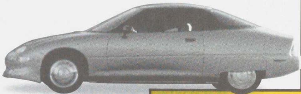
**BODY CONSTRUCTION** Aluminum alloy space frame with aluminum and plastic body panels
