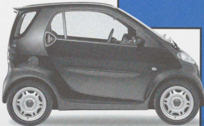
**BODY CONSTRUCTION** Steel space frame with plastic composite body panels
