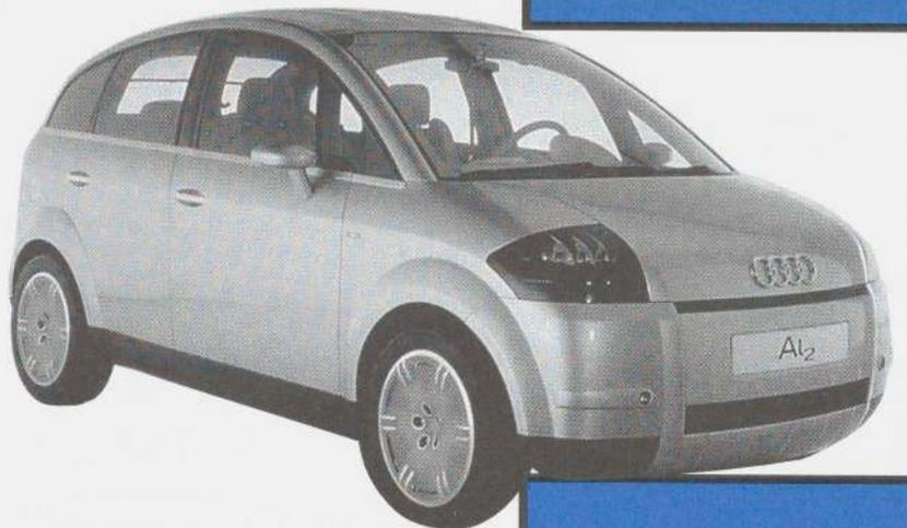
windows supported by light alloy struts. In an attempt to make the car "family friendly," an advanced electronics package includes a steering wheel-based control system, a navigation system, photo-sensors for parking, emergency call, and an automatic distance control that alerts drivers when they are getting too close to the car ahead. A manual gearbox features an automatic clutch.
