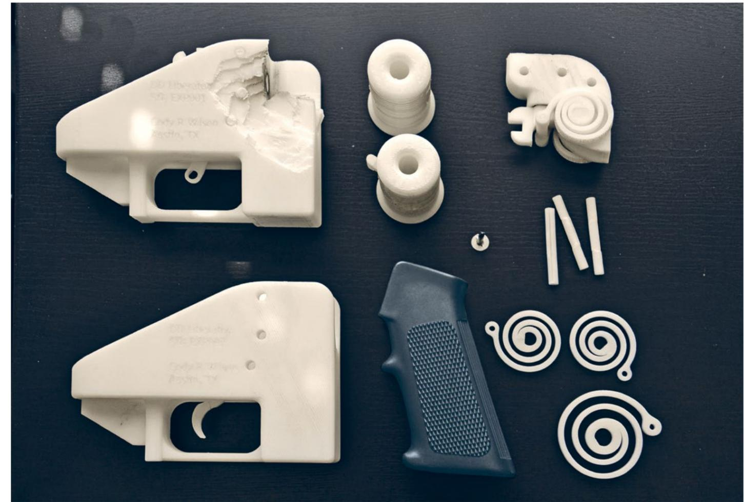
Partial components of The Liberator (clockwise from top left): ABSplus thermoplastic frame, barrel, hammer body, frame pins, springs, grip; aluminum nail (center)
